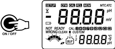
After measurement switch the meter off, clean the electrode and store it with a few drops of HI 70300 storage solution in the protection cap. The auto-off feature turns the meter off after 20 minutes with no button pressed to save battery life. To disable this feature, see "Setup Menu" section on page 9.
