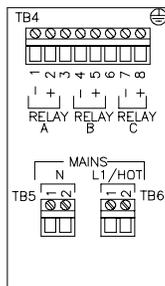
TERMINAL STRIP ARRANGEMENT FOR ANALYZER EQUIPPED WITH A.C. SOLID STATE RELAYS
