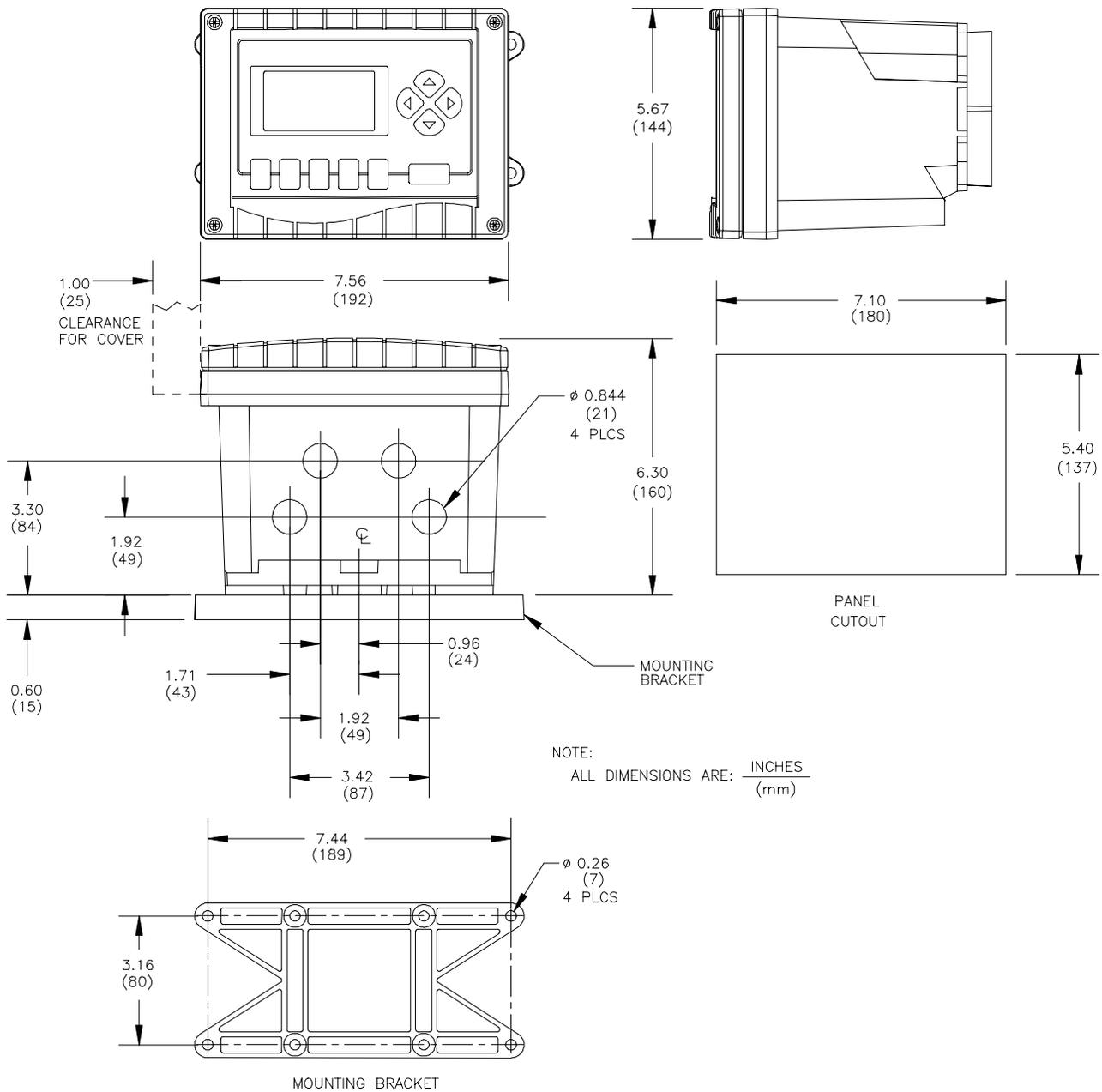
FIGURE 2-2 Analyzer Installation Dimension Details
