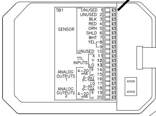
TERMINAL STRIP ARRANGEMENT FOR ANALYZER EQUIPPED WITH ELECTROMECHANICAL RELAYS
