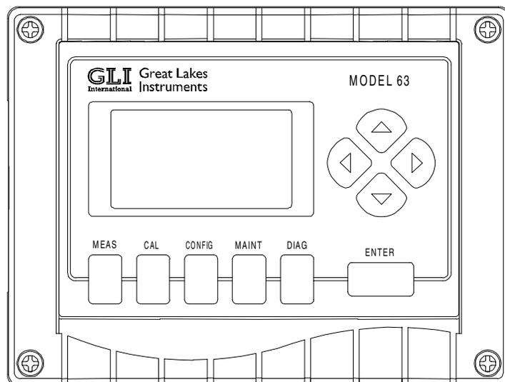
FIGURE 3-1 Analyzer Keypad
