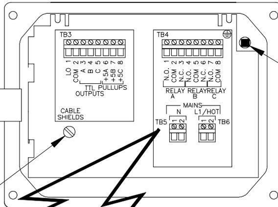
TERMINAL STRIP ARRANGEMENT FOR ANALYZER EQUIPPED WITH D.C. SOLID STATE RELAYS
