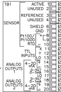
TERMINAL STRIP ARRANGEMENT FOR ANALYZER EQUIPPED TO ACCEPT CONVENTIONAL COMBINATION ELECTRODE OR ELECTRODE PAIR
