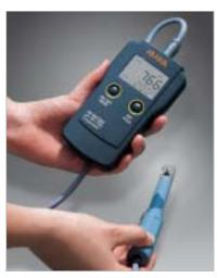
With only two buttons, users can select parameters, calibrate the sensor and change the TDS factor and temperature coefficient (BETA). The multifunctional, industrial probe houses the pH and conductivity sensor along with an integrated solid state amplifier to eliminate noise and interference.
